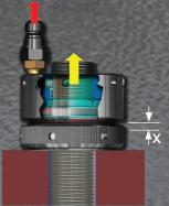
Pressurise the hydraulic nut to the target pressure. The bolt will stretch and a gap will appear at X. Hold the pressure.
