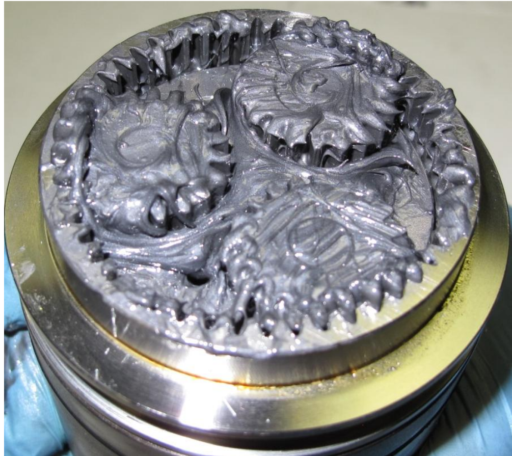
Reference photo of proper amount of grease to apply.
