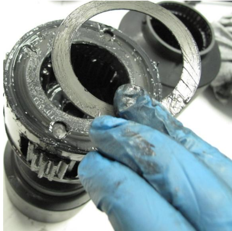
Remove 4 th stage thrust washer. Only on RP-6000
