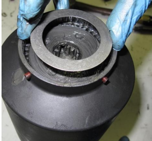
Install 3 rd high speed thrust washer (Only for RP-3000 – Part # RP-30-HSA-TW)
