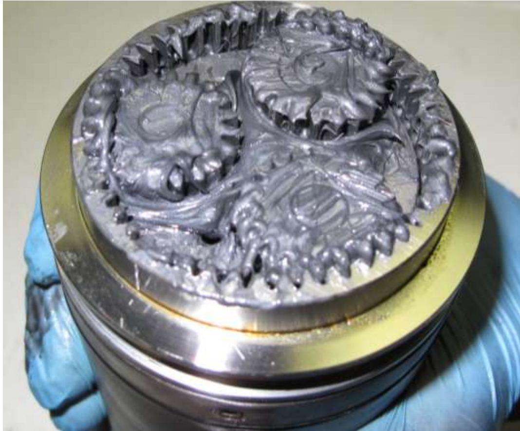
Reference photo of proper amount of grease to apply.
