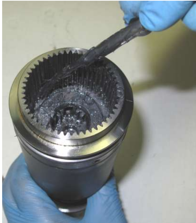
Lightly grease stage gear.
