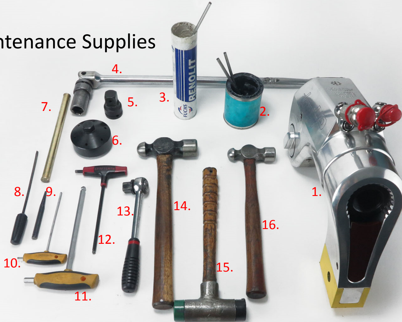
1. TU-20 Cylinder 2. Marine moly 3. Light grease 4. Breaker bar with 7/8" socket 5. 1" square socket 6. TU-20 gland wrench 7. Brass drift 8. Flat tip screw driver 9. Center punch 10. 5/32" allen wrench 11. 3/8" allen wrench 12. 1/4" allen wrench 13. Ratchet 14. Hammer (32oz) 15. Dead blow hammer 16. Hammer (18oz.)
