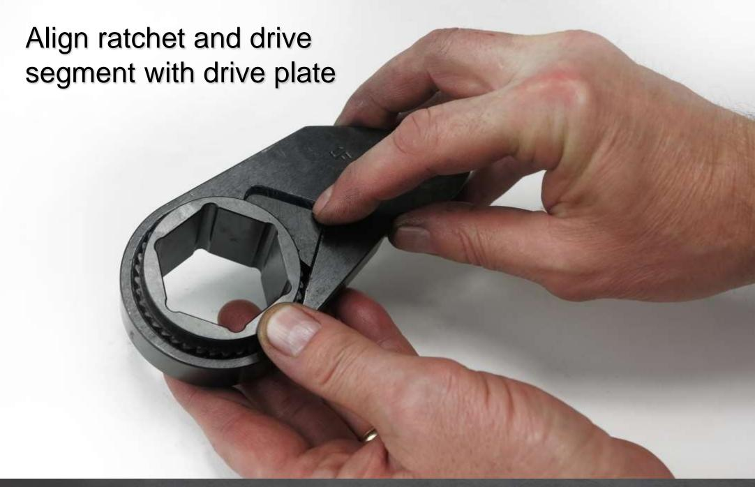
Insert drive segment spring and press into drive plate
