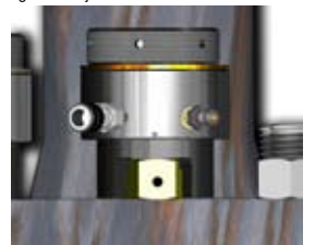
Once the target pressure is reached 'hold' the pressure and rotate the nut back down against the joint face. The bolt is loaded.
