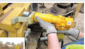
Hyspan PG powered from hydraulics of an excavator.
